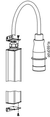
2. Install the PDU to the rack with the provided four (4) M5 x10 mm self-tapping screws.
