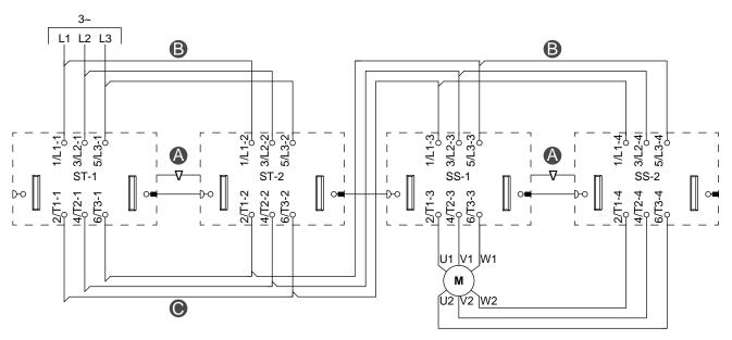
Motor Two Speeds Two Directions - Safe Stop, W. Cat 1/2
