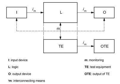
SRP/CS, the safety-related part of the control system, of Wiring Category 2 must be designed so that their function(s) are checked at suitable intervals by the machine control system.
