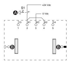
Figure 5 - SIM — Two Channel Wiring
