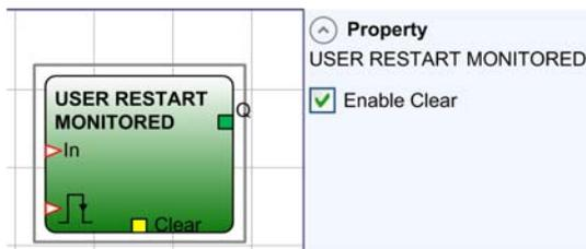
The USER RESTART MONITORED operator is used to save the restart signal according to the following truth table:
