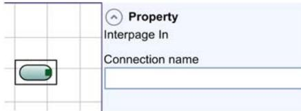
The operator is connected to the input of the function block, for example: `OSSD`. The operator must be given the same unique name as used on the `Interpage Out` operator function block.
