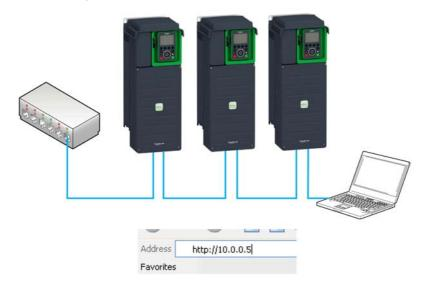
First connect the computer to the drive by typing http:// followed by the drive IP address. You have to enter the **User Name** and a **Password**.
