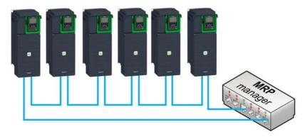
The ring topology can only be used with a media redundancy protocol (MRP) capable managed device. The bus watchdog shall be increased when using MRP function in order to avoid triggering untimely [Fieldbus Com Interrupt] ( $E \cap F$ ).
