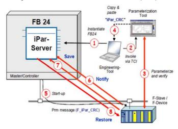
Per upload request, the function block reads the data record with the iParameter out of the drive, creates a data block, and stores the data record therein.
