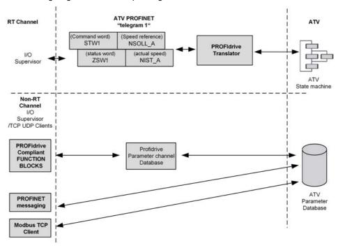
The following section describes how the VW3A3627 is operated when configured in PROFIdrive mode (telegram 1).
