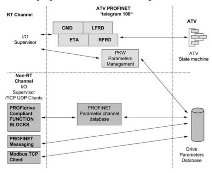
The native mode of the PROFINET VW3A3627 is used when telegram 100 is used.
