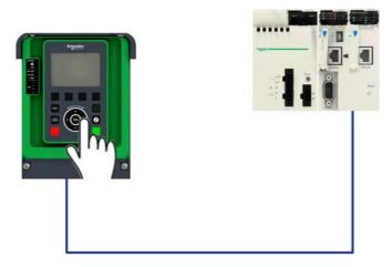
The drive is controlled from the fieldbus (PROFINET) but the reference is adjusted on the controller terminal. The control word comes from the controller and is written according to CiA 402 profile.
