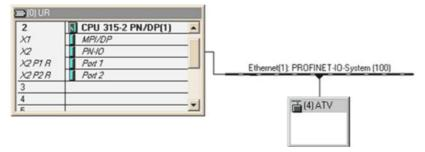
Define the addresses of the cyclic data and PKW data in the PLC periphery:
