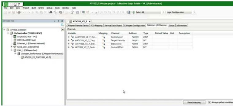
In the **PDO Mapping** tab, configure and activate the PDOs.
