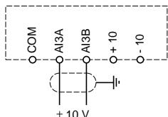
Speed control with tachogenerator feedback
