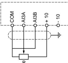
Bi-polar speed reference on a ± 10 V external supply or PI function feedback
