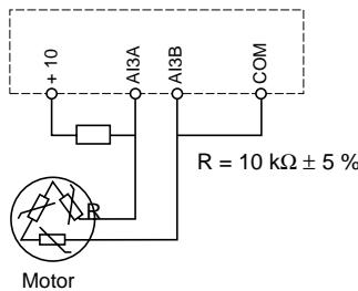
Example of motor switching diagram :
