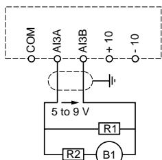
Voltage on the high speed analog input HSP :
