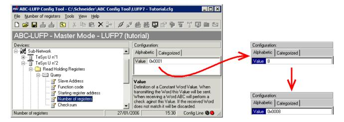
2) Changing the number of data bytes in the Modbus response: The number of bytes read from the "TeSys U n°2" motor starter memory increases from 2 to 16, as the number of registers monitored has increased from 1 to 8. Select the "Byte count" element from the "Response" and change its value as shown below. ABC-LUFP Config Tool will automatically convert any value entered in decimal to hexadecimal.
