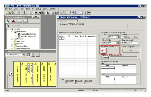
Click on the "hilscher" button (enclosed in a red box above) to start the SyCon configuration tool.
