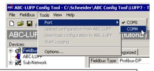
**NOTE**: If all the serial ports of your PC are already used by other applications, you must first close ABC-LUFP Config Tool, then "free" a serial port by disconnecting, closing, or terminating an application that currently uses a serial port. Afterward, restart ABC-LUFP Config Tool because COM ports are only scanned during its start-up; the freed COM port should now be useable by it.
