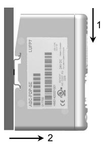
Start by pushing the gateway downwards (1) to compress the gateway's spring. Then pull the bottom of the gateway box forwards (2) until the box comes away from the rail.
