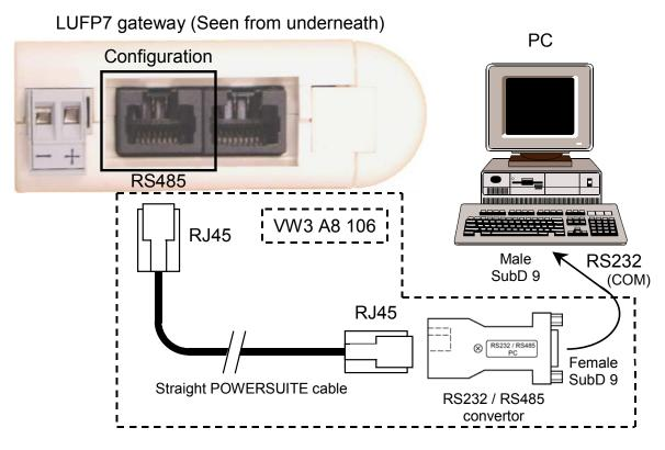
Once the gateway has been connected to a PC with the PowerSuite cable and the RS232/RS485 converter, you can change its configuration using "ABC-LUFP Config Tool". This configurator also allows you to carry out a few diagnostics on the gateway.
