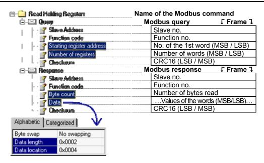
**NOTE:** In all cases, the "Query / Slave Address" and "Response / Slave Address" elements are automatically updated by ABC-LUFP Config Tool according to the node in which the command is located. Their values cannot be changed by the user. In the same way, the "Query / Function code" and "Response / Function code" fields depend on the nature of the Modbus command and cannot be changed by the user.
