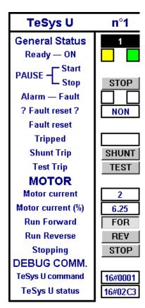
The "Sr0" sub-program is called once per motor starter from the "Cmd\_mon" program. Each of these calls should be made with a different value in the word %MW0 (between 0 and 7) as it is used to index the status word and the command word of the same motor starter. The sub-program assists the screen presented on the previous page in conducting the following tasks:
