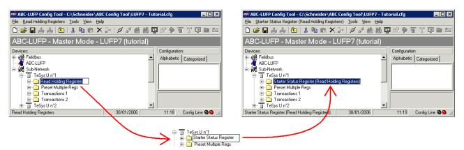
This renaming function can also be used for the Queries and Responses of the Modbus Commands and Transactions, as illustrated by the following example:
