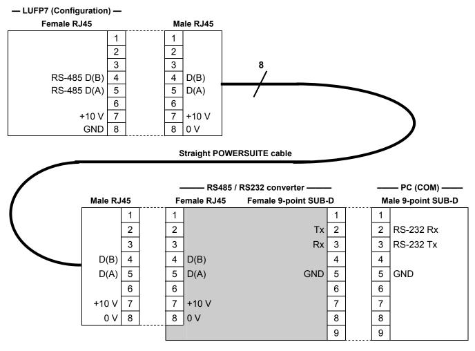
**NOTE:** The inversion of the Rx and Tx signals between the gateway and the PC is shown on the 9-point SUB-D connectors, because beyond this junction, the RS-232 signals are replaced by the D(A) and D(B) polarizations of the RS-485 signals.
