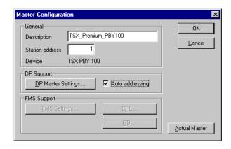
Lastly, select the Profibus-DP master and run the "Bus Parameter..." option from the "Settings" menu to configure the Profibus-DP network baud rate.
