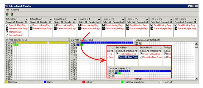
To see which memory locations are occupied by data from the command you are interested in, uncheck the box corresponding to the "Preset Multiple Registers" command from the "TeSys U n°4" node, as shown above. We can see that the Modbus data transmitted with the query corresponding to this command occupy 2 bytes located from address 0x0208.
