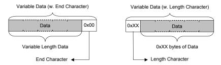
The end / length character of any "Variable Data" located in the Queries of Transactions must be supplied by the Profibus-DP master because it is the producer of this data.
