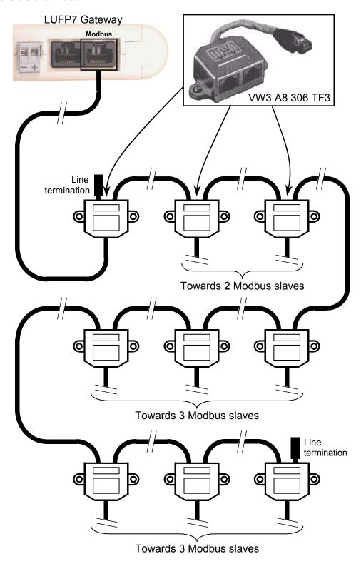
"Bus" topology with SCA junction boxes: This topology is similar to the previous one, except that it uses TSXSCA62 subscriber connectors and/or TSXCA50 subscriber connectors. We recommend using a VW3 A68 306 connection cable and the TSXCSA•00 Modbus cables. Connect the RJ45 connector on the VW3 A68 306 cable to the Modbus connector on the LUFP7 gateway.
