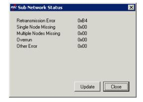
**NOTE:** The "Sub Network Status" window may be useful to detect problems on the Modbus sub-network. So, if the number of retransmission errors increases upon using the "Update" button, this denotes the absence of one or more slaves, Modbus cabling or speed problems, or invalid Commands and/or Transactions. Since retransmission errors tend to lower the general performances of the Modbus communications, you should undertake actions to prevent these retransmission errors from increasing!
