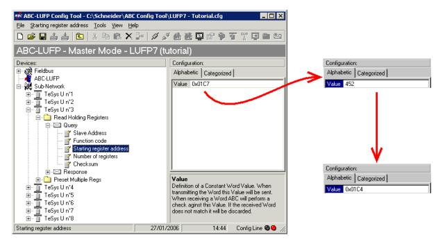
This operation in no way changes the content of the gateway's memory, because we do not need to change the values of the "Data length" and "Data location" fields of the "Data" element of the "Response" to the aforementioned command. So no additional operations will be necessary, either in ABC-LUFP Config Tool, or in SyCon.
