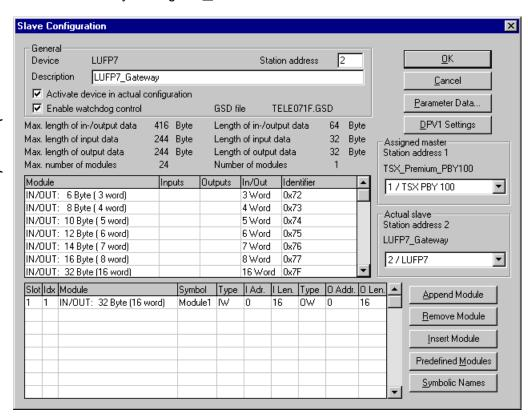
**NOTE:** Do not use the "Symbolic Names" option to name the I/O exchanged with the gateway. This operation is useless because the symbols you shall define under SyCon would not be exported and retrieved under PL7 PRO.
