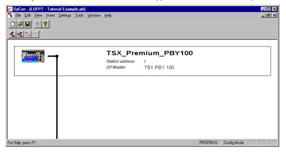
Double-click on the line that corresponds to the Profibus-DP master to open the "Master Configuration" window.
