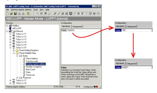
This operation in no way changes the content of the gateway's memory, because we do not need to change the values of the "Data length" and "Data location" fields of the "Data" element of the "Query". So no additional operations will be necessary, either in ABC-LUFP Config Tool, or in SyCon.
