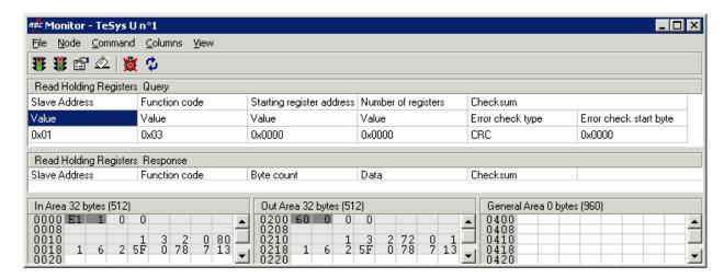
The upper part of this window allows you to choose a Modbus command, to edit its contents, then to send it to the Modbus network ("Command" menu). The response will then be displayed in this same part. Please see chapter 2.10 Node monitor in the ABC-LUFP Config Tool user manual, entitled **AnyBus Communicator – User** for further information about how to use this window.
