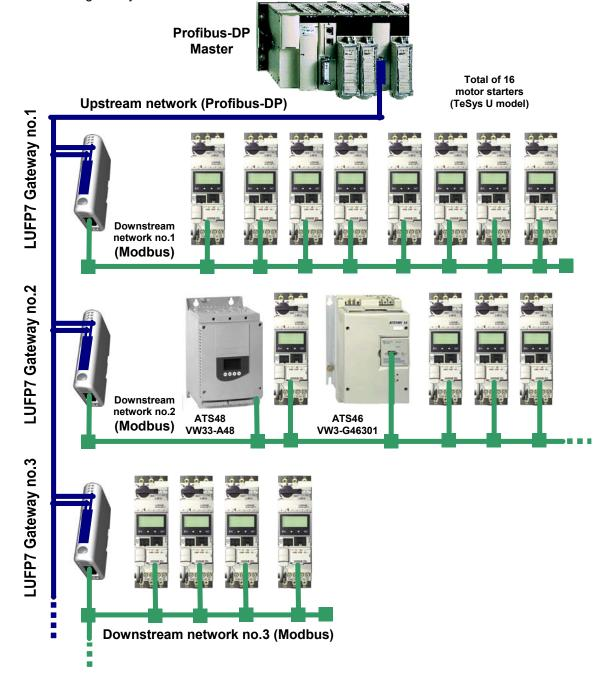
The LUFP7 gateway behaves both as a Profibus-DP slave on the upstream network and as a Modbus RTU master on the downstream network.
