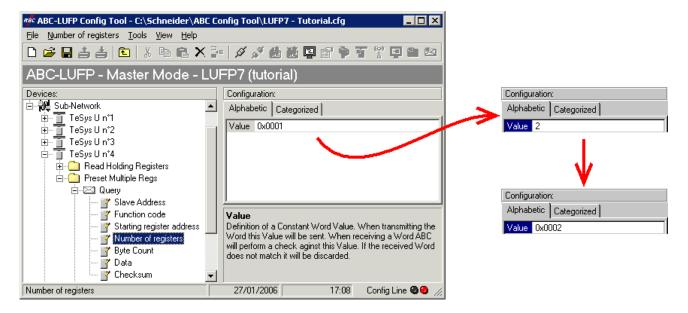
2) Changing the number of data bytes in the Modbus query: The number of bytes written into the memory of the "TeSys U n°4" motor starter memory increases from 2 to 4, as the number of registers controlled has increased from 1 to 2. Select the "Byte count" element from the "Query" and change its value as shown below. ABC-LUFP Config Tool will automatically convert any value entered in decimal to hexadecimal.
