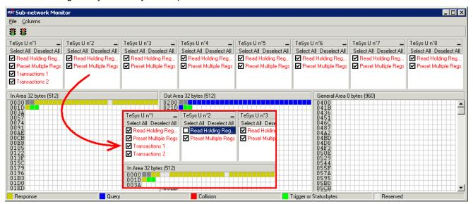
To see which memory locations are occupied by data from the command you are interested in, uncheck the box corresponding to the "Read Holding Registers" command from the "TeSys U n°2" node, as shown above. We can see that the Modbus data received in response to this command occupy 2 bytes located from address 0x0004.
