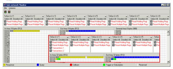
You will note that the "TeSys U n°1" section now only has the two Modbus commands common to the eight TeSys U motor starters, and that the memory locations which corresponded to the two personalised commands are now free.
