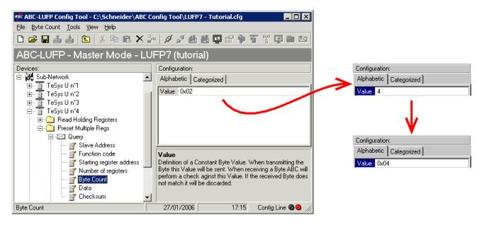
3) Changing the location of the Modbus data transmitted into the gateway's memory: As the number of bytes written (see previous step) has increased from 2 to 4, the Modbus data to be transmitted to the "TeSys U n°4" motor starter must be placed at a different location in the gateway's memory, and the size of the memory occupied must also be adjusted appropriately.
