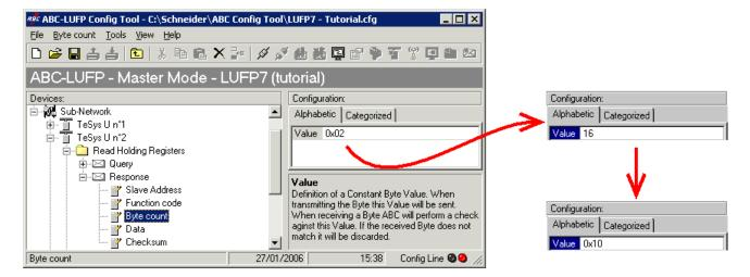
3) Changing the location of the Modbus data received in the gateway's memory: As the number of bytes read (see previous step) has increased from 2 to 16, the Modbus data received must be placed at a different location in the gateway's memory, and the size of the memory occupied must also be adjusted appropriately.
