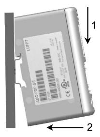
Start by fitting the rear base of the gateway to the upper part of the rail, pushing downwards (1) to compress the gateway's spring. Then push the gateway against the DIN rail (2) until the base of the gateway box fits onto the rail.
