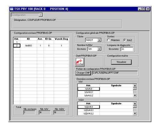
If you use the vertical sliders in the "PROFIBUS-DP slave data" frame, you can see that the gateway's 16 input words have been allocated to inputs %IW4.0 to %IW4.0.15 and that its 16 outputs words have been allocated to outputs %QW4.0 to %QW4.0.15.
