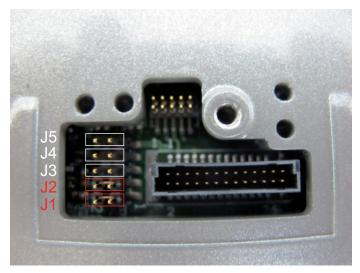
Connect the optional module DIS1 by inserting it into the contact pins, as shown in the following figure.
