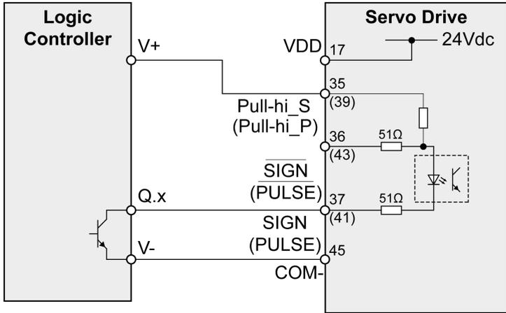
Pulse Input (Open Collector, Positive Logic)
