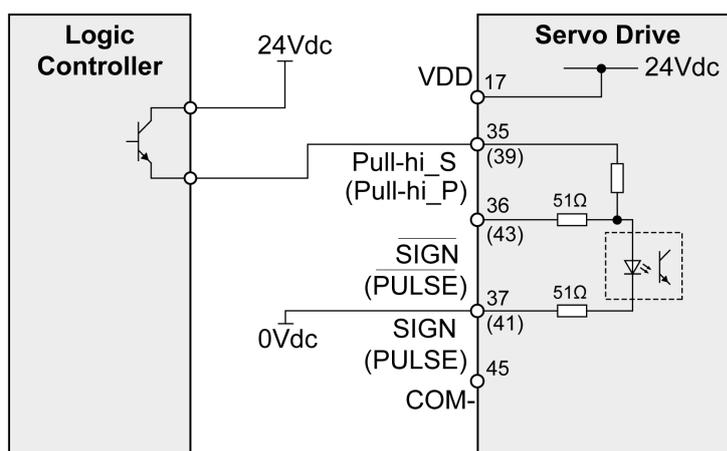
Example of pulse input (open collector) with external power supply (positive logic).
