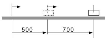
In the case of an absolute movement, the movement is absolute with reference to the zero point.
