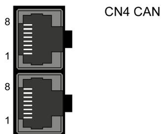
The CAN interface (CN4) consists of 2 RJ45 connectors. The following table describes the contacts of the connectors:
