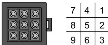
Encoder connection MIL connector (Type B), motor side:
