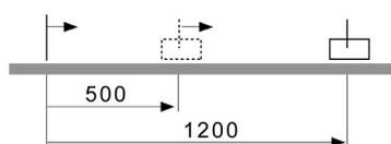
Homing or position setting is required before the first absolute movement can be performed.
