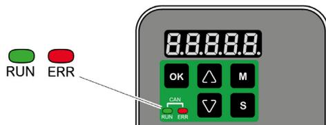
The illustration below shows the signals of the CAN bus status LEDs (Run=GN; Err=RD).
