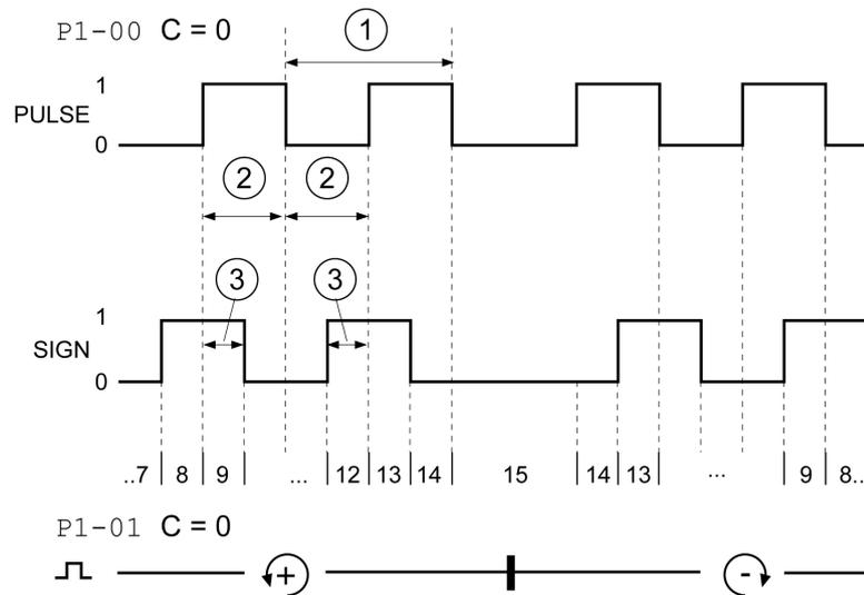
The signal shape shown relates to the factory setting (P1-00 C=0). The direction of movement shown relates to the factory setting (P1-01 C=0).
