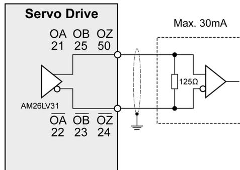
Example of encoder output signal, high-speed optocoupler.
