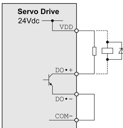
Example of digital outputs DO1 ... DO5 with external power supply (negative logic):
