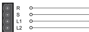
Wiring diagram logic supply LXM28A••M3X
