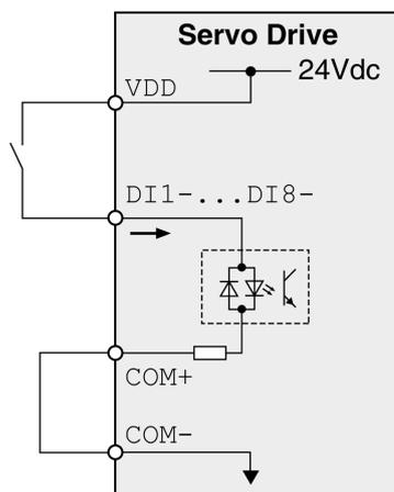
Example of digital input with external power supply (positive logic):
