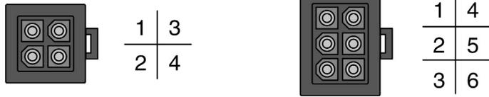
Motor connection MIL connector (type C and type D), motor side:
