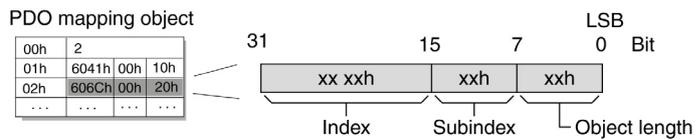
Subindex 00<sub>h</sub> of the communication object contains the number of valid subindex entries.
