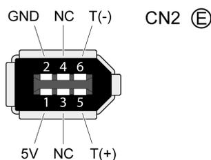
The motor encoder interface (CN2) is a 6-pin connector. The following table describes the contacts of the connector:
