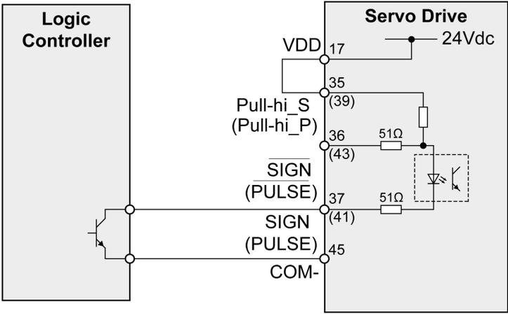
Example of pulse input (open collector) with external power supply (negative logic).
