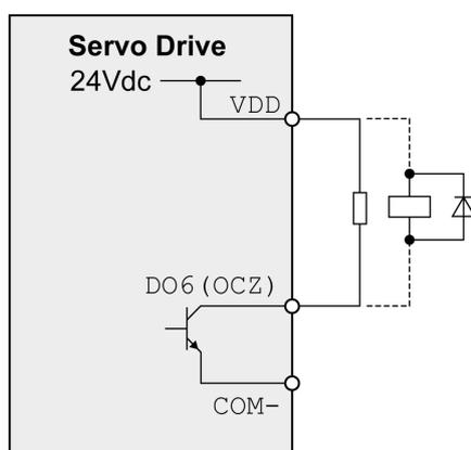
Example of digital output DO6 (OCZ) with external power supply (negative logic):
