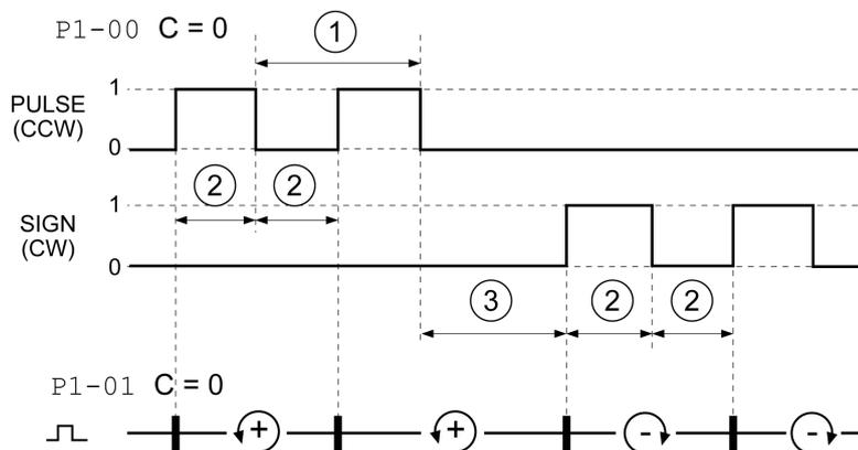
The signal shape shown relates to the factory setting (P1-00 C=0). The direction of movement shown relates to the factory setting (P1-01 C=0).
