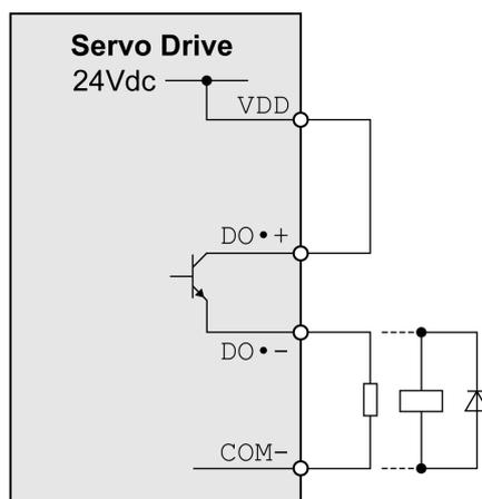
Example of digital outputs DO1 ... DO5 with external power supply (positive logic):
