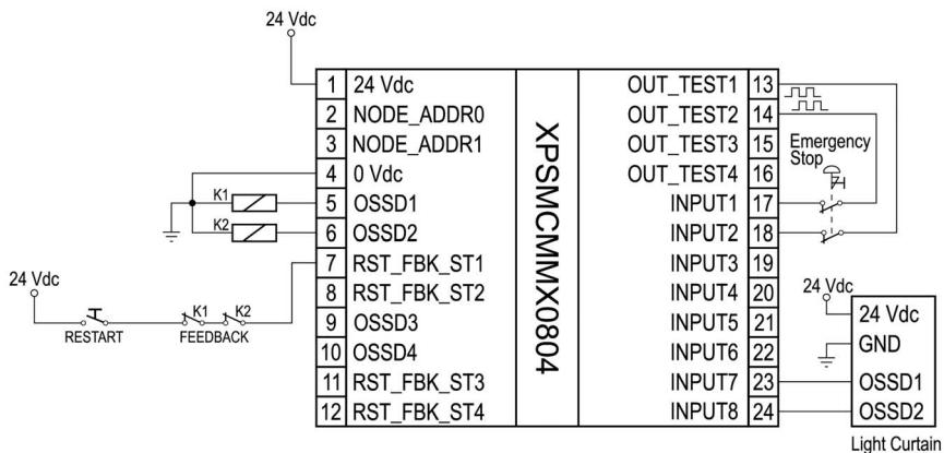
**NOTE:** Best practice dictates the use of fusing on the incoming 24 Vdc power, and sized appropriately for the requirements of the module.
