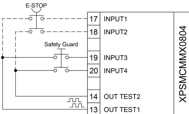
Interface Type C, class 3 according to "ZVEI CB241 Ed.2" with a maximum test pulse duration of 100 µs.
