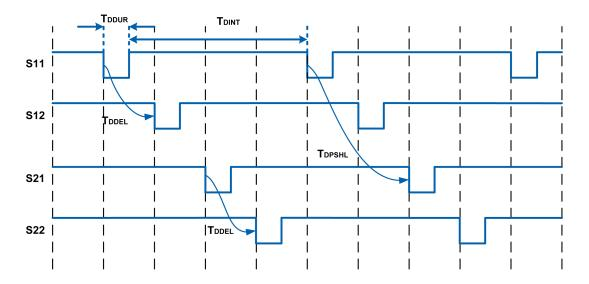
The diagram presents the input channels S11-S12 and S21-S22. The remaining input channels S13 and S23 as well as the remaining safety-related inputs S31-S32-S33, S41-S42-S43, S51-S52-S53, and S61-S62-S63 use the same logic as the input channels and safety-related inputs illustrated.
