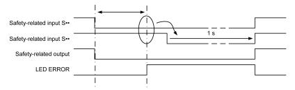
The first safety-related input is deactivated which starts the signal interlock monitoring time of 200 ms. The second safety-related remains activated longer than 200 ms. This triggers a signal interlock alert 200 ms after interlock monitoring has started.
