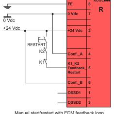
Manual start/restart with EDM feedback loop
