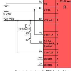
Manual start/restart with EDM feedback loop
