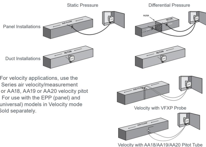
Note: For velocity applications, use the VFXP Series air velocity/measurement probe or AA18, AA19 or AA20 velocity pitot tubes. For use with the EPP (panel) and EPU (universal) models in Velocity mode only. Sold separately.
