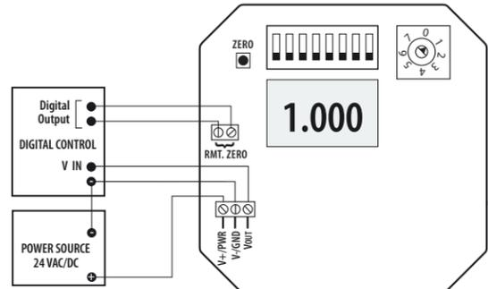
9. Wait five seconds, then press and hold the ZERO pushbutton for two seconds or provide contact closure on the AUX ZERO terminal. This will reset the output and display to zero pressure. For best accuracy, press the ZERO button while both ports are open to atmospheric pressure. To protect the unit from accidental zero, this feature is enabled only when the detected pressure is within about 0.5 in. WC (125 Pa) of factory calibration.
