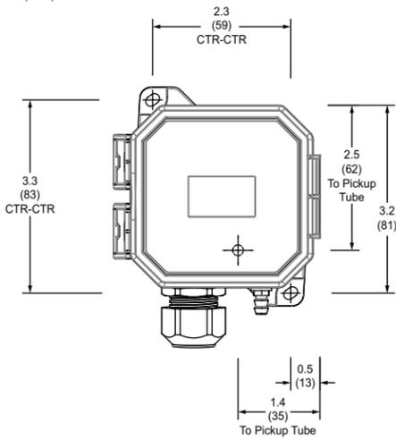
5. For applications using conduit, remove the cable gland nut on the bottom of the unit. Thread a standard 1/2-in. NPT female threaded coupler onto the body of the cable gland. Connect the opposite end of the coupler to the conduit.
