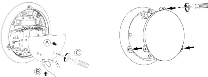
For side cable entry, use the knockouts provided in the luminaire base. In order to ensure the luminaire is sealed, it is vital to use the cable grommets.
