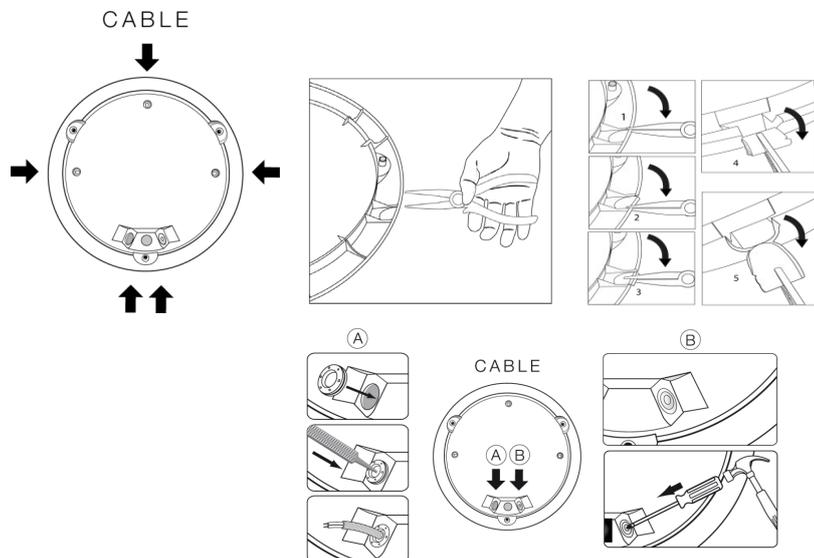
For side cable entry, use the knockouts provided in the luminaire base. In order to ensure the luminaire is sealed, it is vital to use the cable grommets. Use 1.5 mm<sup>2</sup> U1000R2V type cable (recommended to maintain sealing). Use a pointed object to pierce the centre of a cable grommet. Do not use a blade, which might weaken the grommet and impair sealing. Fit the grommet into the cable entry and feed the supply cable through it.
