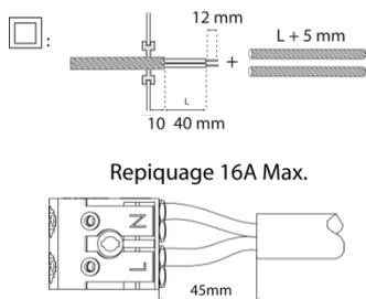
The cable must be prepared as per the diagrams. The conductors must be stripped for a length of 12 mm. The protective sleeves supplied with the kit must be threaded onto the wires, to comply with the Class II requirements. Respect the polarity.
