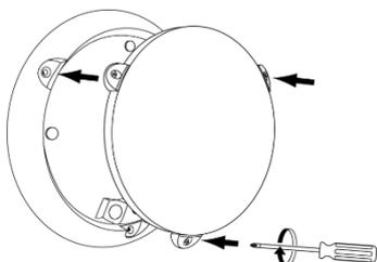
Tighten the 3 diffuser fixing screws + the screw covers on the diffuser using a suitable screwdriver and the **98000003** vandal-resistant bit.
