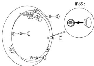
For mounting the luminaire, use 5 mm diameter flat-headed screws with fixing plugs suitable for the type of wall, in order to achieve optimum rip-out resistance. The screws and plugs are not supplied with the luminaire. Fit the 4 blanking plugs in order to maintain the sealing of the product.
