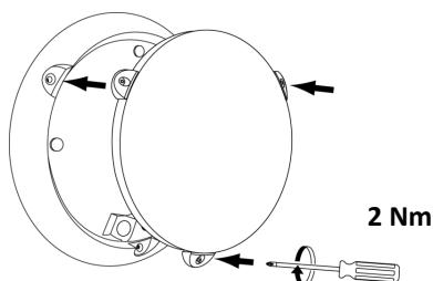
For side cable entry, use the knockouts provided in the luminaire base. In order to ensure the luminaire is sealed, it is vital to use the cable grommets. Use 1.5 mm<sup>2</sup> U1000R2V type cable (recommended to maintain sealing).
