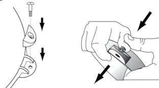
Fit the 3 screws cover and clip the screws onto the diffuser.
