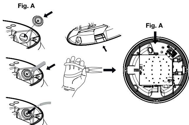
For side cable entry, use the knockouts provided in the luminaire base. In order to ensure the luminaire is sealed, it is vital to use the cable grommets.
