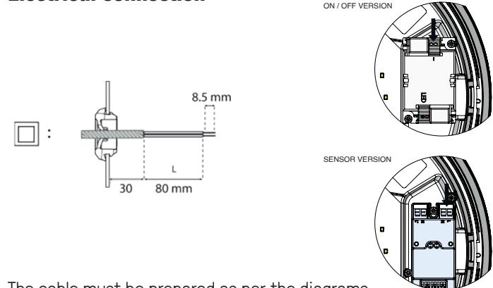
The cable must be prepared as per the diagrams.
