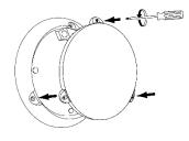
For side cable entry, use the knockouts provided in the luminaire base. In order to ensure the luminaire is sealed, it is vital to use the cable grommets.
