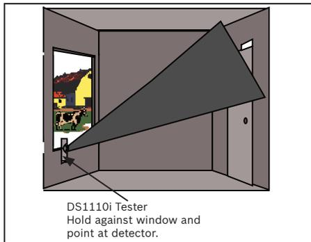
Figure 7.1: Test #2 Response Test
