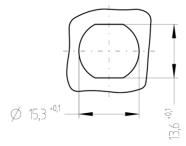
Tin cut-out for torsional protection
