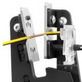
Stripping the insulation material off with the blades
