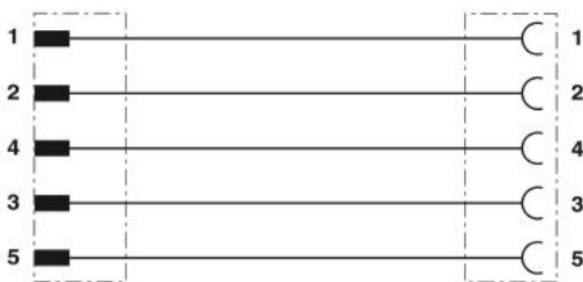
Pin assignment between M12-plug and M12-jack
