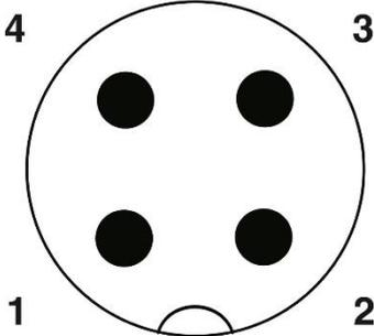
Pin assignment M12-plug, 4-pol, A-coding
