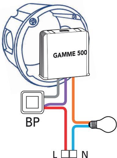
**CABLAGE EN 2 FILS A LA PLACE D'UN ALLUMAGE VA-ET-VIENT**
