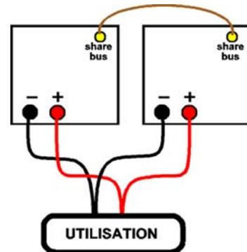
The recommended wiring for paralleling is the following :
