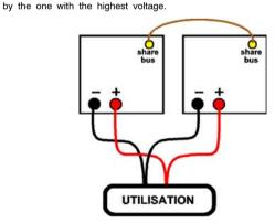
The recommended wiring for paralleling is the following:
