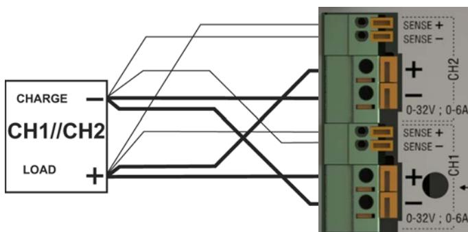
Tracking mode coupling (symetric)
