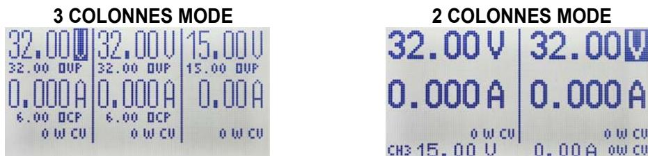
Since the outputs are on that " ON " measurement Voltage and Current is displayed instead of the set if different. Simply touch on V or A selection keys, displays the operator instructions.
