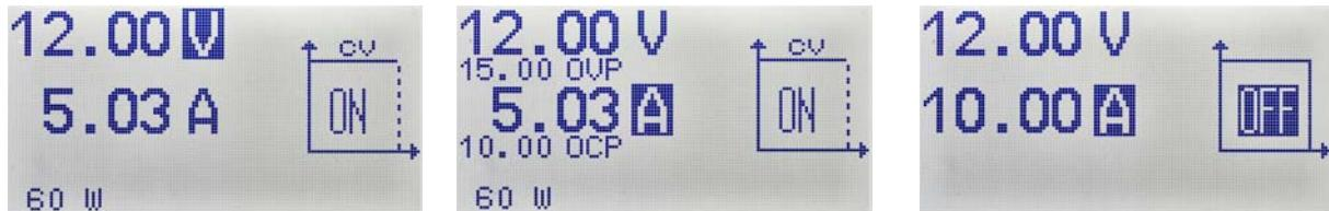
The measurement (voltage or current) is displayed instead of the set, if different. Simply touch on V or A selection keys, displays the operator instructions.
