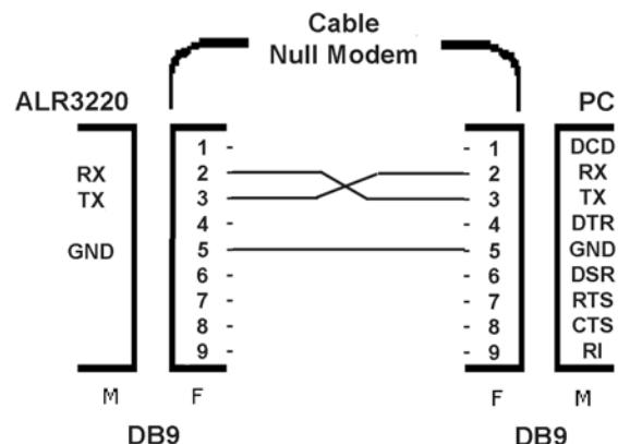
Connect power supply to the serial port of the PC using an RS232 cable "null modem" (cross-connections).
