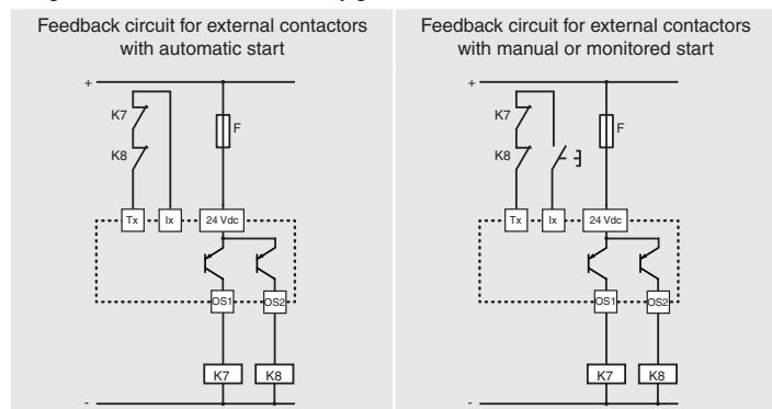
In order to function correctly, any modules or PLCs connected to the OSx safety electronic outputs must be able to withstand cyclical deactivation tests performed on the same.
