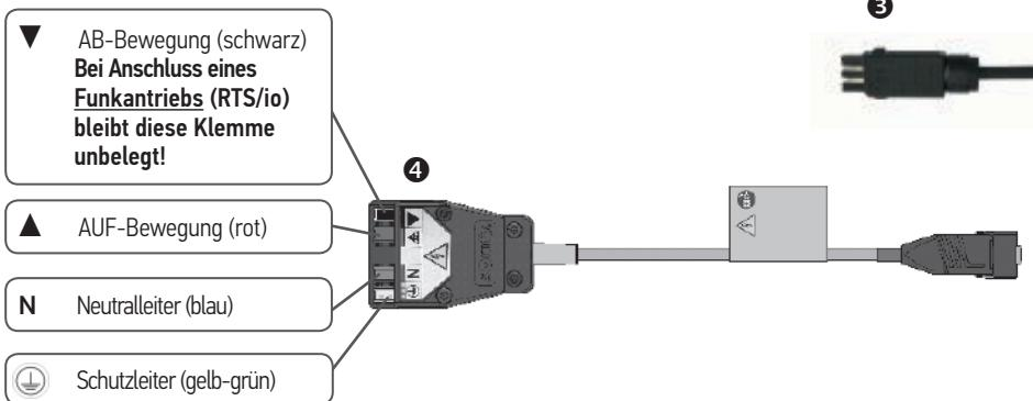
**4.2. io HYBRID-ANTRIEBE:** io HYBRID Setting Cable Kit 9020579
