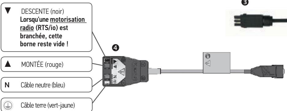
**4.2. Motorisations io HYBRID :** io HYBRID Setting Cable Kit 9020579
