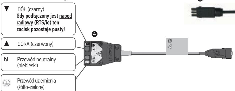
**4.2. Napędy io HYBRID:** io HYBRID Setting Cable Kit 9020579
