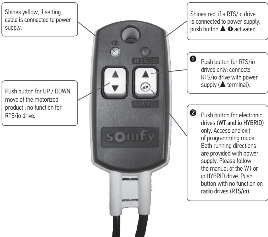
**⚠** The push buttons **▲ ①** and **▼ ②** must **not** be activated with the following motors: LS, LT, LT PA, Orienta motors, J41TN/2TN/HTM (damage can be caused to!).
