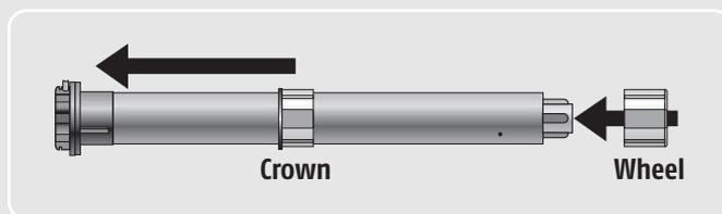
The crown is placed on the tubular motor head and the wheel is on the opposite side, on the output shaft. Both the crown and the wheel are specifically designed to the size and the shape of the tube. The wheel drives the tube and so supports the torque, this is the reason why we advise to rivet the wheel to the tube.
