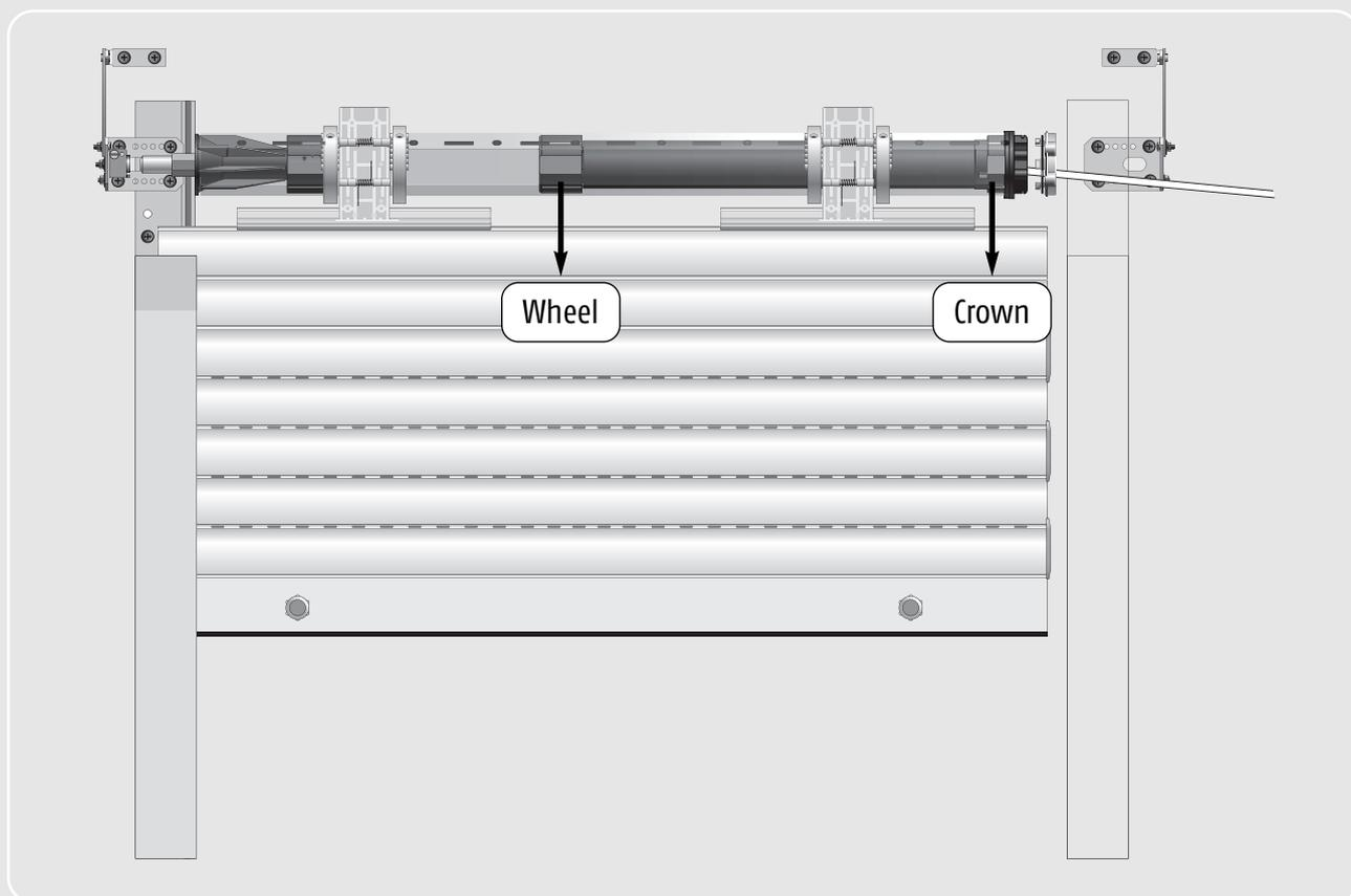
***When using an extruded wheel, a stop wheel is required !!***
