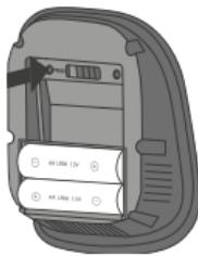
Approach the front panel of the radio receiver's thermostat, and briefly press the "PROG" button situated on top of the thermostat's battery compartment. While searching for the receiver, the thermostat's blue and red LEDs will flash quickly. Wait for a few seconds.
