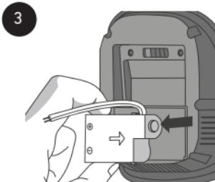
Remove the power supply module from the thermostat's front panel.
