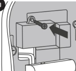
Refit the terminal block protective guard, and screw it back down.
