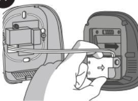
Clip the io thermostat power supply module onto the thermostat's front panel.
