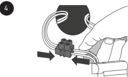
Connect the thermostat's power supply module cables to the power supply cables leading from the recess box, using an appropriate connector.
