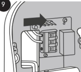
Insert the cables and clip them onto the NO & COM outputs of the automatic clip terminal block (no polarity).
