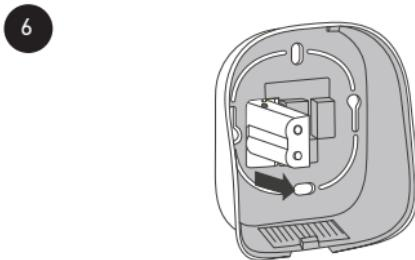
Feed the thermostat's power supply module through the orifice on the thermostat's rear panel.
