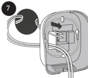
Feed the boiler control cables (NO / COM) through the rear panel.
