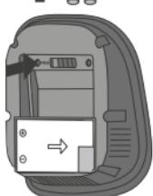
Briefly press the "PROG" button located on top of the battery compartment of the thermostat. While searching for the receiver, the thermostat's blue and red LEDs will flash quickly. Wait for a few seconds.
