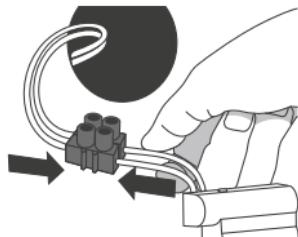
Connect the thermostat's power supply module cables to the power supply cables leading from the recess box, using an appropriate connector.
