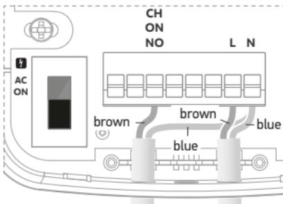
**Installation for NO floor heating:** Connect the receiver's NC & N terminals (NB: an NO valve is connected to the NC terminal in the receiver). Then connect these 2 cables to the valve NO. Then connect the brown cable to the L terminal block for live, and the blue cable to the neutral N. Connect the other end of this second cable to the switchboard (L to live & N to neutral). Finally, set the switch on the receiver to the AC ON position.
