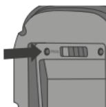
If you do not complete pairing within this period, use a pointed object to press on the PROG button on the back of the thermostat's front panel for 3 seconds. Make sure that the power supply module remains in place when removing the front panel from the thermostat.
