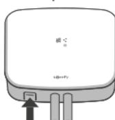
Press and hold the receiver's "PROG" button for 3 seconds to pair a boiler, heat pump, floor heating or pilot wire radiator. The "Connection" LED will begin to flash green, and pairing mode will be active for 10 minutes. If you want to pair an independent hot water tank, press and hold the Prog button for 6 seconds; the green LED will flash again.
