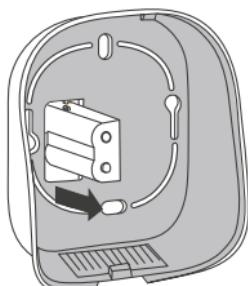
Feed the thermostat's power supply module through the orifice on the thermostat's rear panel.
