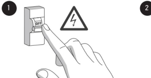
Switch off the power supply before starting to install the io thermostat.
