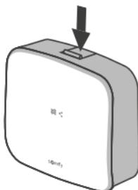
As far as possible, avoid installing the receiver too close to the body of the boiler or any other metal object that could interfere with the radio waves. It is advisable to mount the radio receiver on the wall in the area surrounding the heating appliance so that the controls are accessible (PROG button + indicator light).
