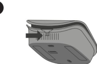
Unclip the front panel from the rear panel by pressing on the pressure point.
