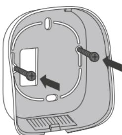
Fasten the rear of the io thermostat using the screws from the flush-mounting box or the screws and plugs provided
