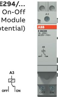
By snapping on an E294/... Central On-Off Control Module at the Main Module E290, it's not allowed to use an E292/... contact module or an E299/... auxiliary contact!
