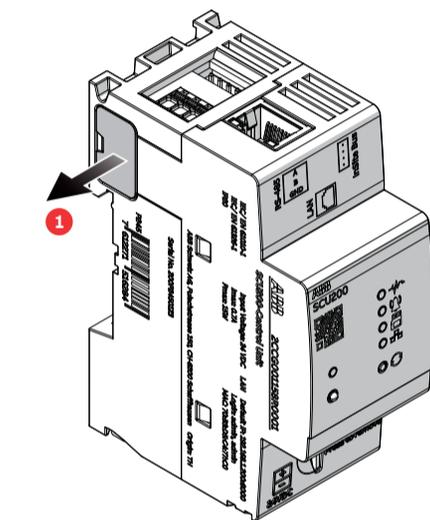
and insert the connector plug placed on the right side of the InSite expansion module. Pay attention to the correct interlocking between modules.
