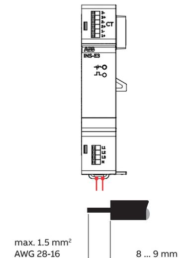
Connect the number of phases desired to the voltage measurement inputs. It is desirable to use L1 & N for one phase network and L1, L2, L3 & N for three phase with neutral network.
