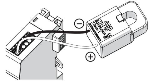
**Attention:** Ensure correct cable placement of the current transformer by connecting the black cable to the '-' terminal and the white cable to the '+' terminal and twist the cable.
