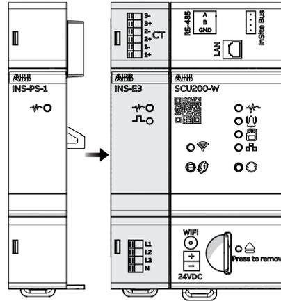
**Attention:** In case one or more expansion modules have to be added to SCU200 / SCU200-W plug them all first before assembling on DIN-Rail bar.
