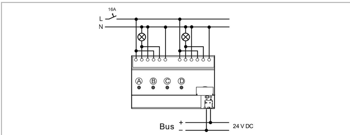
Fig. 12: Example of connection: Channel bundling, two channel respectively (A and B / C and D) connected in parallel
