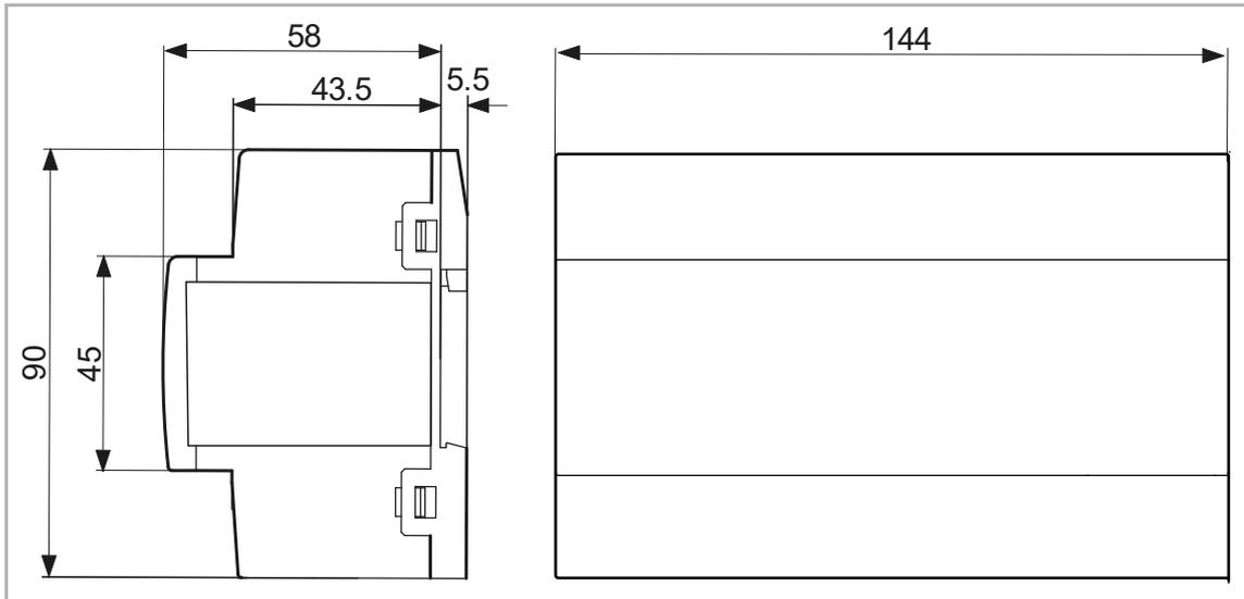
Fig. 7: Dimensions (8 MW)
