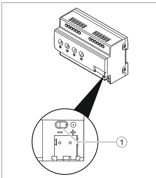
Fig. 17: Programming button (Example: 4gang)
