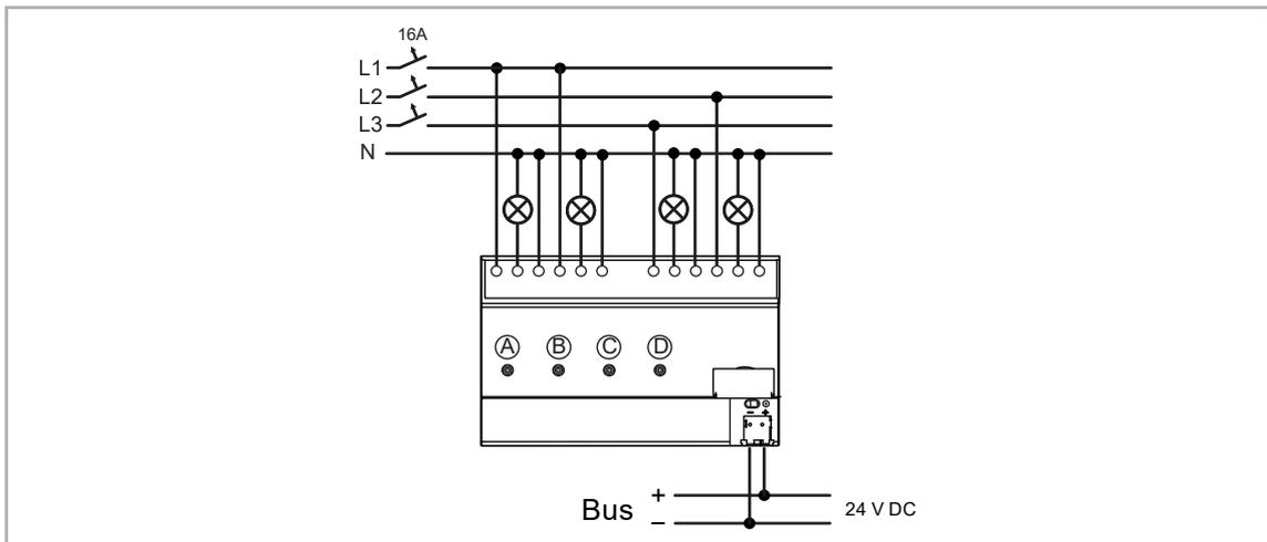
Fig. 13: Example of connection: Multi-phase operation, multi-channel dimming actuator
