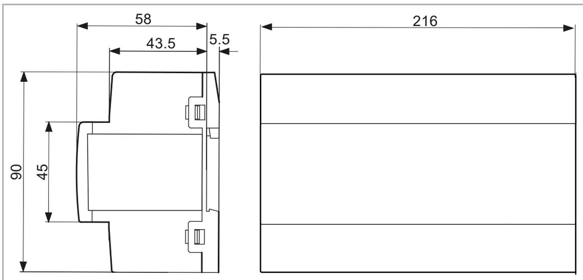
Fig. 8: Dimensions (12 MW)
