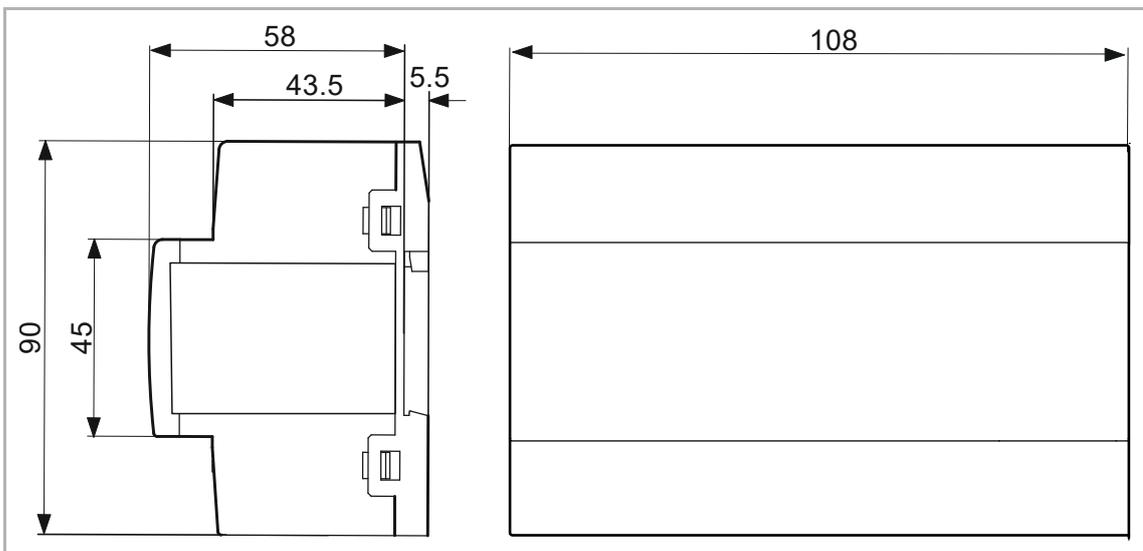
Fig. 6: Dimensions (6 MW)
