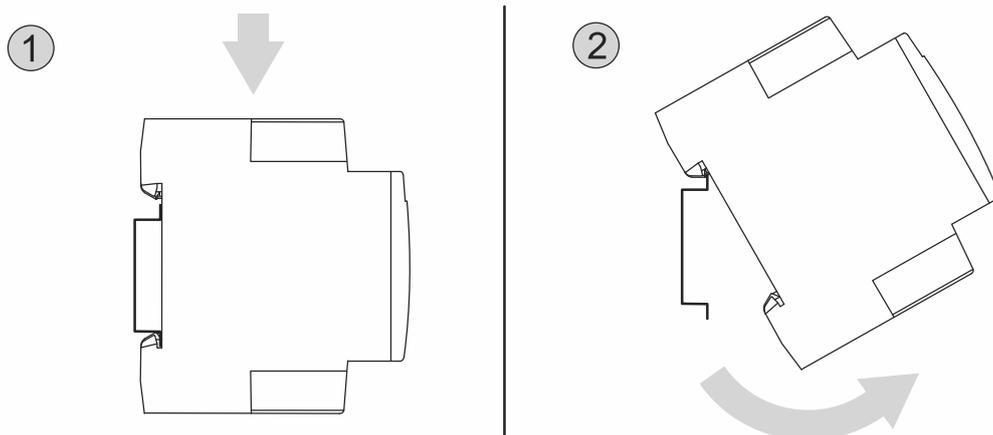
Fig. 10: Removal from the mounting rails
