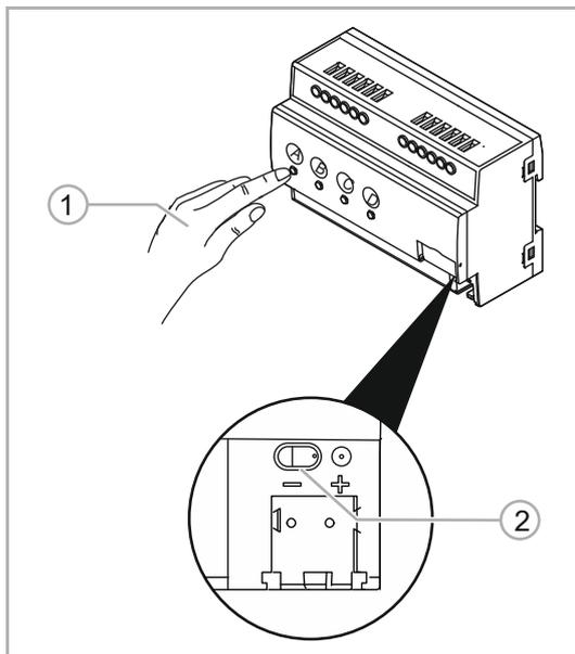
Fig. 18: Control elements (Example: 4gang)
