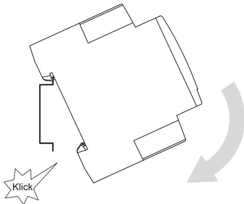
Fig. 9: Installation on mounting rails
