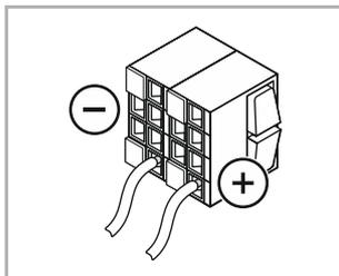
Fig. 14: Connecting terminal KNX
