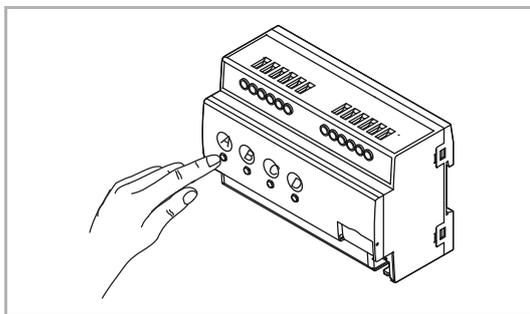
Fig. 20: On-site operation on the device (Example 4gang)
