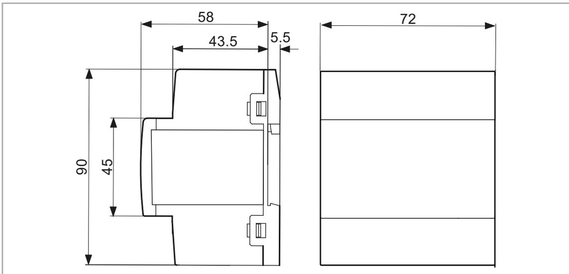
Fig. 5: Dimensions (4 MW)
