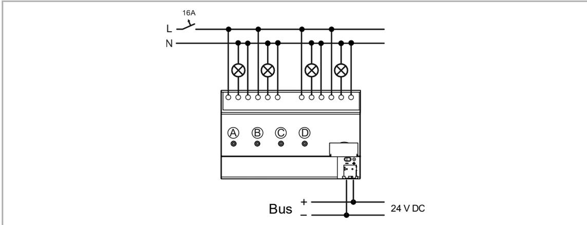
Fig. 11: Example of connection: Single-phase operation, multi-channel dimming actuator
