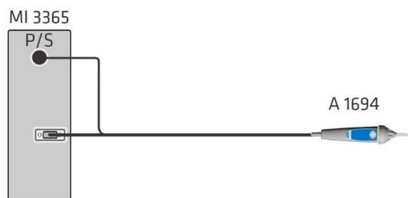
Figure 9.3: Raccordement du Tip Commander (A 1694)
