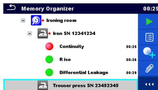
Figure 5.5: Status - Measurements completed with fail result(s)
