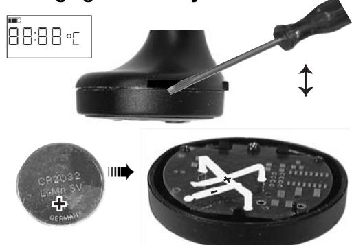
The battery has to be changed if appears in the display during the measurement. Open the housing using a screwdriver. Remove the used button cell.
