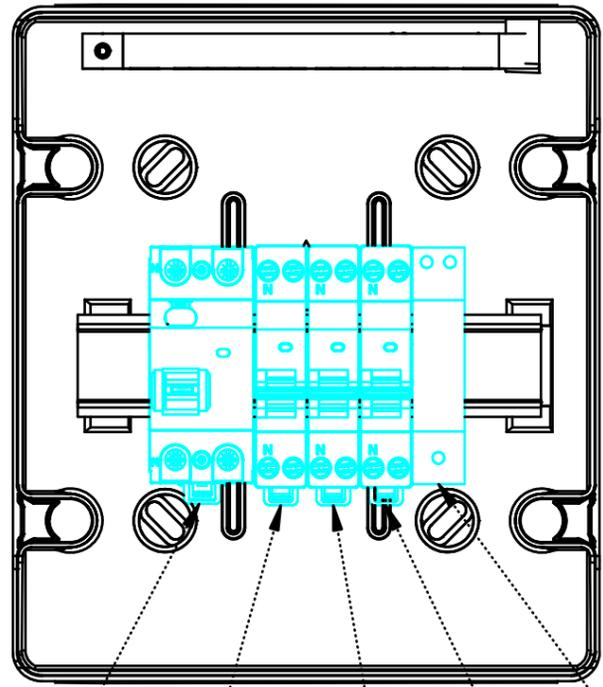
INTER DIFFERENTIEL PROTECTION ONDULEUR 1 PROTECTION ONDULEUR 2 PROTECTION PARAFONDRE PARAFONDRE
