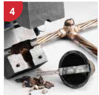
4 Open the mold and remove the expended steel cup – no special disposal required
