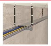
To help ensure the availability and operation of safety systems after an earthquake event, many building and industry codes now include requirements for the design and installation of seismic sway bracing for non-structural components, such as fire sprinkler, mechanical, electrical and plumbing systems.
