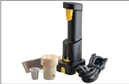
Fig. 2 – Prepare the proper materials and equipment for the type of connection you are making. The Cadweld Plus One Shot system requires a Cadweld One Shot ceramic mold, Cadweld Plus welding material, wire brush for cleaning/preparing conductors, nVent ERICO Cadweld Plus Impulse Exothermic Welding Control Unit, and propane torch.
