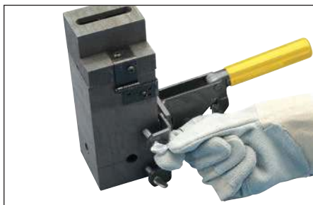
Fig. 7 – Tighten the clamp thumbscrews onto the mold.
