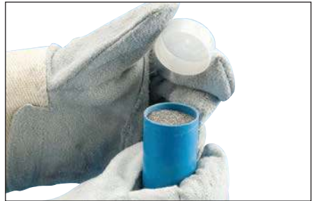
Fig. 19 – Remove the lid over the mold crucible.
