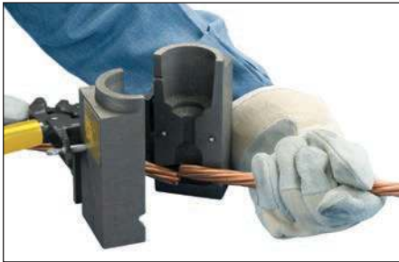
Fig. 15 – Insert the conductors and position them for the connection.
