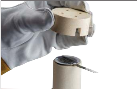
Fig. 10 – Place the ceramic lid onto the mold.
