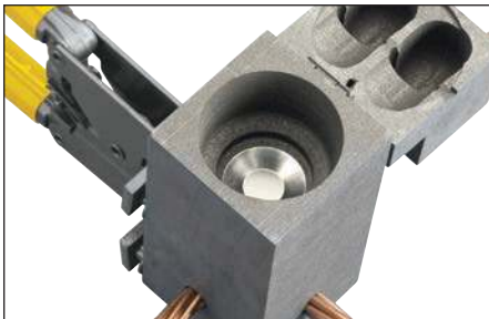
Fig. 17 – Ensure that the steel disk is properly seated.
