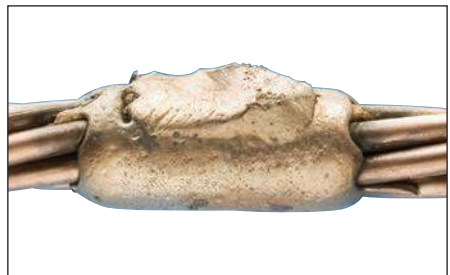
Fig. 29 – Completed Cadweld connection.
