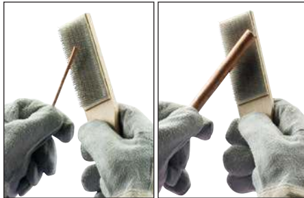
Fig. 5 – Next, use a wire brush to further prepare the surface of the conductors and ground rod (nVent ERICO T-313 or T-314 brush). Scrape the outer surface to remove dirt and oxidation. You will notice a slight color change.
