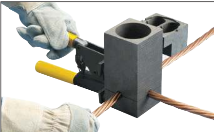
Fig. 13 – Insert the conductors and position them for the connection.
