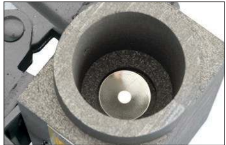
Fig. 19 – Ensure that the steel disk is properly seated.
