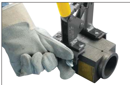
Fig. 7 – Tighten the clamp thumbscrews onto the mold.
