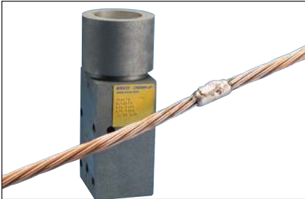
Fig. 31 – Ready to make another Cadweld connection.
