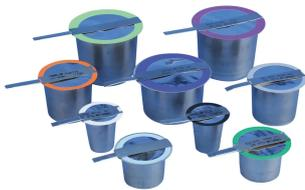
nVent ERICO Cadweld Plus Welding Material, F20, allows for an expedited, permanent grounding connection using pre-measured, self-contained cups. Each package of welding material can be easily placed into the mold and safely ignited with the nVent ERICO Cadweld Plus Impulse Exothermic Welding Control Unit to create an irreversible bond.
