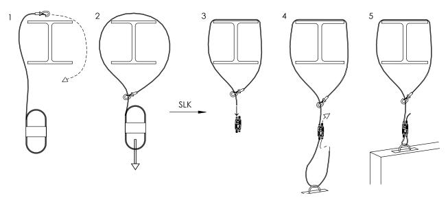
The process illustrated above shows proper installation when wrapping Speed Link with a Hook End-Fitting around a beam. Installing Speed Link this way will allow the installer to have the height adjustability at the load (easier than having it at the structure).
