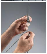
STEP 4: Insert wire rope back into locking device.
