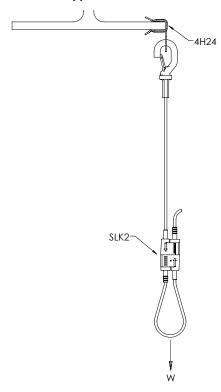
By attaching to structure with another nVent CADDY product, the height adjustment of the system is moved on the end of the rope that is closer to the load. This makes it much easier to make fine height adjustments because installers do not have to estimate the amount of rope that needs to be added or removed at the structure. It is also much easier for the installer to lift the application at the load and adjust the wire.
