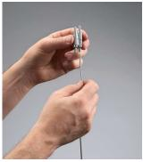
**STEP 2:** Insert wire rope into I ocking device.
