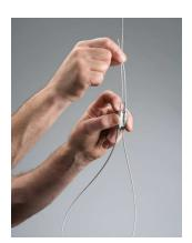
STEP 1: Pinch the free end of the cable against the loaded cable above the locking device. This will provide a temporary support for the load and hold the position of the cable. Meanwhile, grip the locking device firmly and push down on the release tube on the loaded side of the cable.
