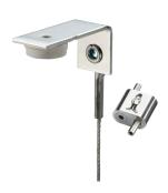
The nVent CADDY Speed Link Light Pack with Nail Gun Bracket includes a precut length of 1mm wire rope riveted to an angle bracket designed for direct fastening together with an ultra-low-profile locking device. Contractors can quickly and safely install it to the concrete ceiling using a wide range of nail guns to support and secure lighting and signage.
