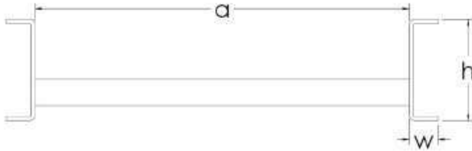
Figure 8: Cable ladder cross-section with basic dimensions
