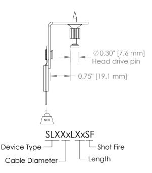
Uses Powers Fasteners, Inc. part number 50032. For minimum fastener embedment depths in steel or concrete, please consult www.powers.com.
